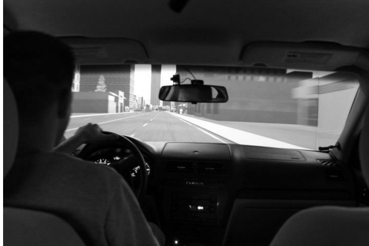
Figure 2: View of Realtime Technologies Inc. Driving simulator from inside of the car.
