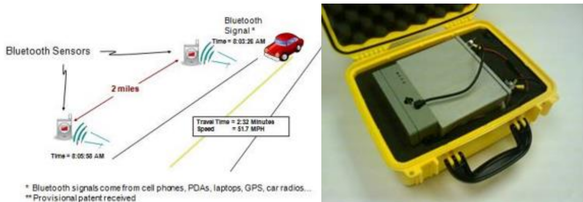
Figure 2 The BluFAX Concept & Device
